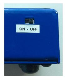
You can disable the switchbox through a switch on the back panel (next to the 25 pin connector).
