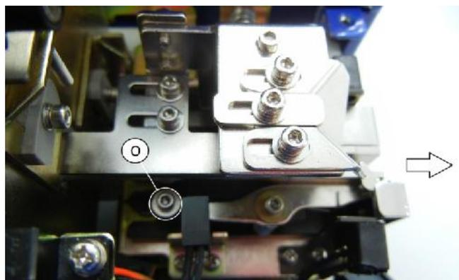
After removing the track and choosing the 2 spacers suitable to the screw used, loosen **P** and **Q** screws, and unscrew **R** screw.
