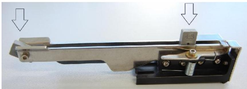
Reassemble the track, tighten **O** screw and closed the gates through **M** and **N** screws, clearance of 1 mm. Tighten **i** and **L** screw.
