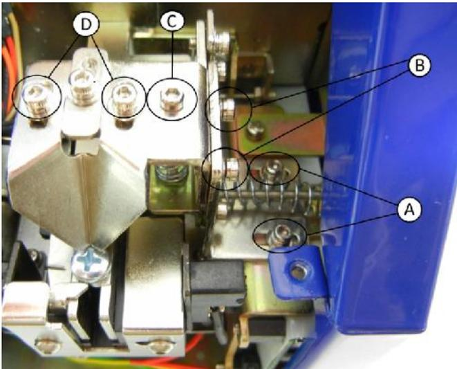
To adjust the height of the block track cover-bit guide, loosen **B** and **C** screws and turn the screw clockwise to lower, and counterclockwise to raise it. Once you have found the right spot tighten **B** screws.
