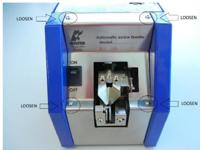
To adjust the bit guide right/left, loosen **A** screws and turn **E** screw: clockwise to move the bit guide to the right, and counterclockwise to move it to the left. Once you have found the right spot, tighten **A** screws.
