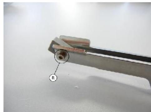
Replace the spacer and tighten the screw **R** starting the new one at an angle of about  $30^\circ$ . At the same time enter the second spacer at end of the track as a reference for the distance between the two plates, then tighten **P** and **Q** screws.
