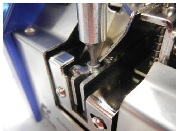
To adjust the height of the track cover/bit guide block, loosen **C** screws through **D** holes.
