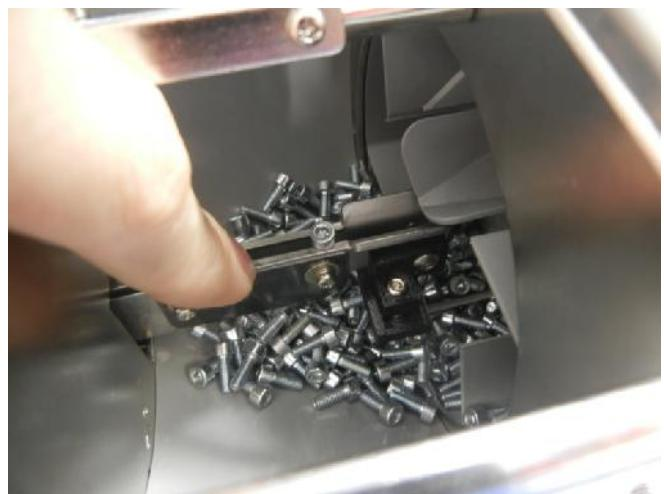
Tighten **H** and **L** screws. Slide a screw through the track: if it should not flow smoothly, repeat the procedure.
