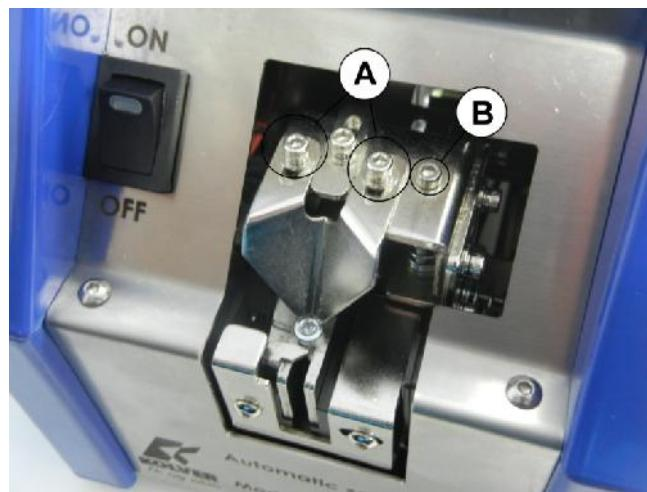
Turn the **B** screw clockwise to decrease or counterclockwise to raise it. Once you have found the right spot, fix **D** screws.
