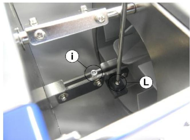
Bring near the 2 sides of the track with the help of your fingers until you find the correct distance of 0.3/0.5 mm larger than the diameter of the screw.
