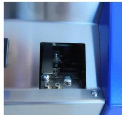
The jack power connector will give a relay contact: open contact is case of missing screw and closed contact in case of screw loaded.
