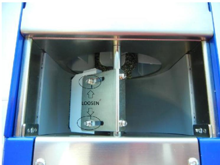
If the brush has been set too high, screws in the wrong position could pass and stop the passage. If too low, the brush could get stuck.
